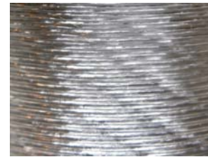
Figure 6. Simple moiré pattern by helical 3D printing
