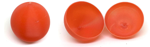
Fig. 1 Example of procedurally 3D-printed empty sphere (surface and inside).
