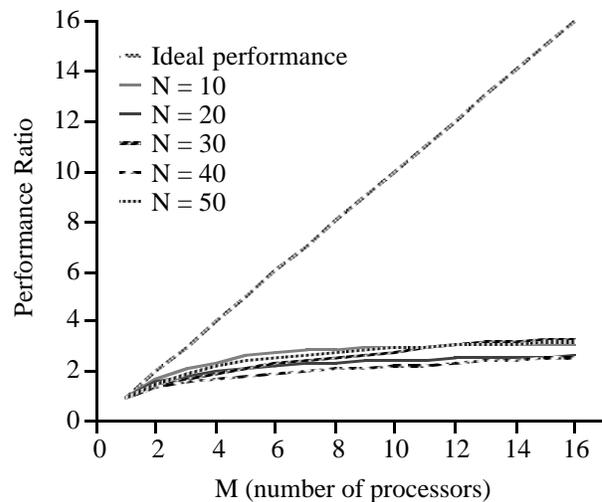
**Figure 11. Simulated performance of the  $N$  queens problem using a less local rule**
