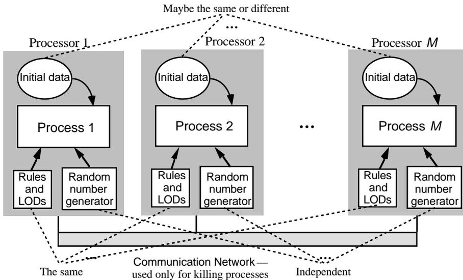
**Figure 7. The method of parallel processing CCM-based computation**
