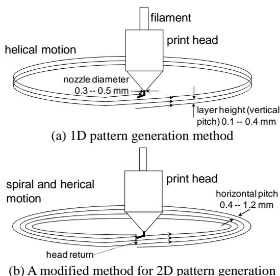
**Fig. 2.** 1D/2D pattern generation method
